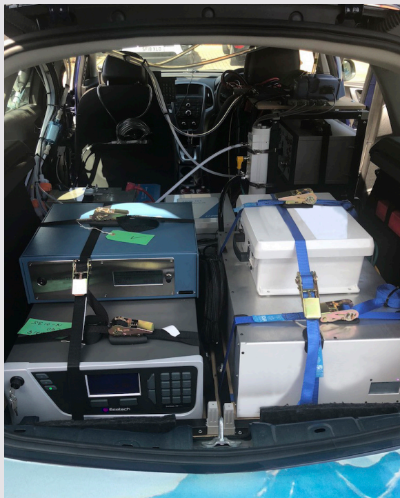
Locked and loaded! Inside a Google Street View car. ECOTECH Serinus® 40 NO x gas analyser pictured bottom left.
